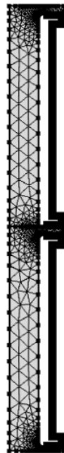
Figure 3.19: Simulation mesh defining solution points for simulation. The figure shows two adjacent LSC's.
