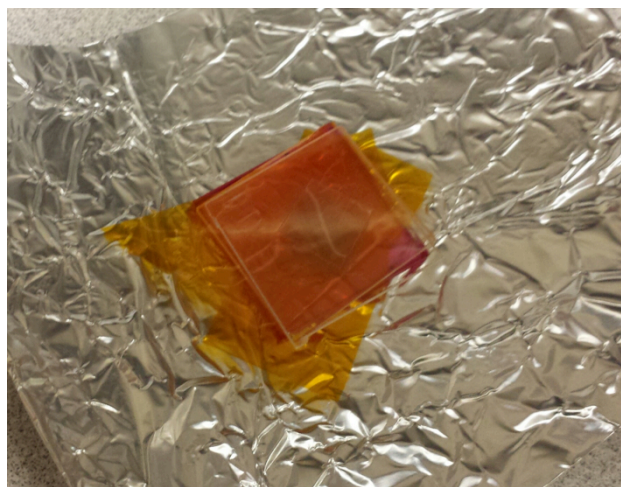
Figure 4.27: Stack of test samples used with Fluorescein sample in middle of the stack, being shielded from other effects.
