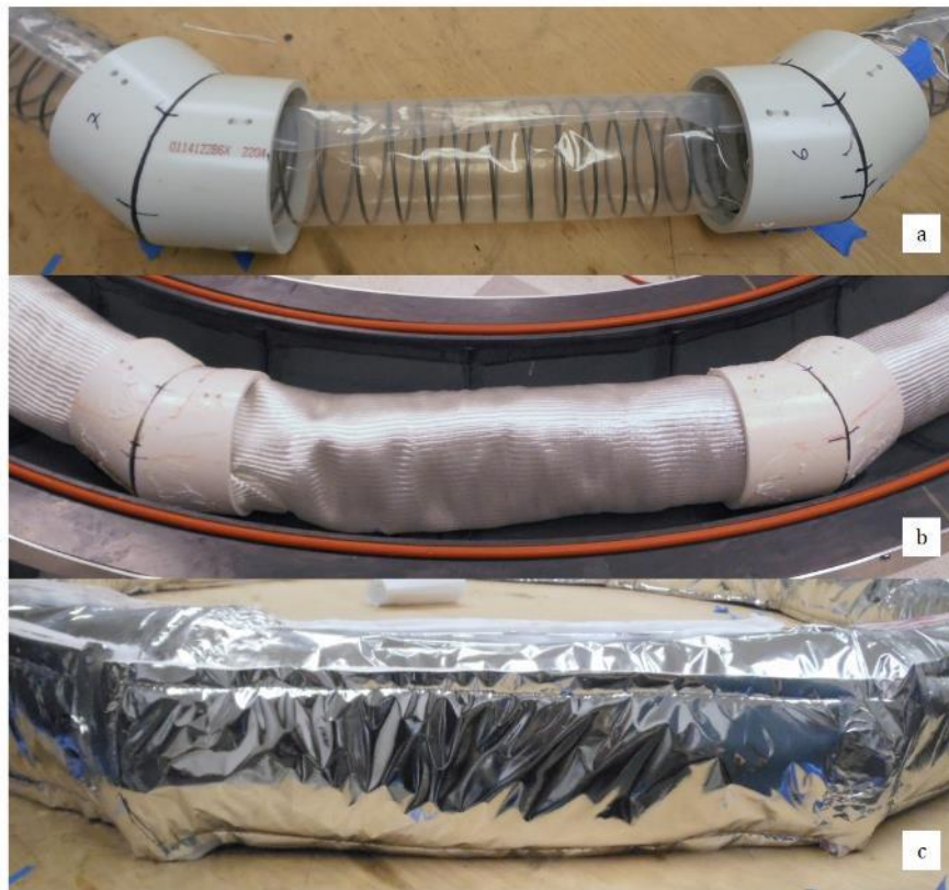
Figure 2.10 Close-up of toroidal enclosure segment with a) inner core, b) fiberglass sleeve over core, c) thermal blanket
