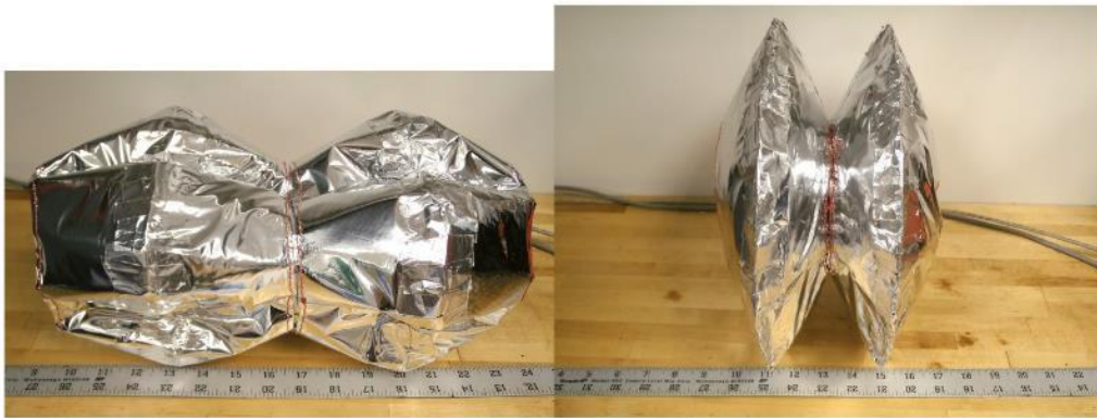
Figure 2.14 Initial concept for accordion-inspired MLI folding
