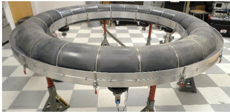
Figure 3.1 Vacuum chamber used for thermal testing
