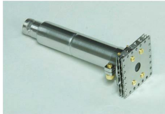
Fig. 44: Kimball Physics FC-71 A Faraday Cup w/energy analyzing grids [50]
