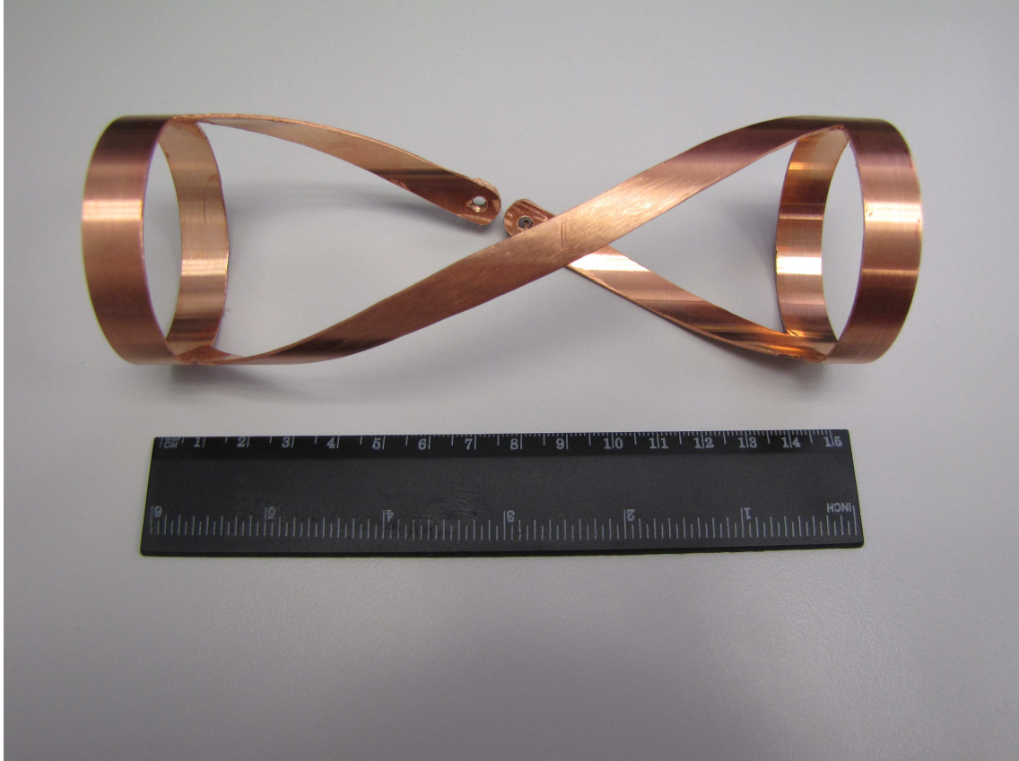
Figure 4.3: 15.4 cm length copper helical antenna.
