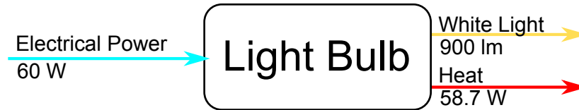
Figure 3.1: Component resource flow example. The lamp shown is a sink for electrical power, and a source for light and heat, each of the quantities shown in the figure.
