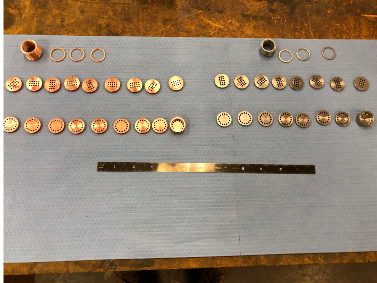
Figure 4.16: Comparison between copper (left) and stainless-steel (right) heat exchangers
