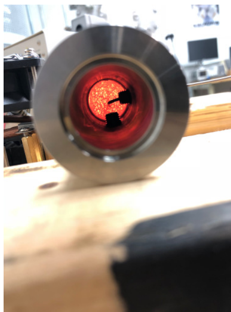
Figure 4.7: Copper metal foam being heated inside the low carbon steel
