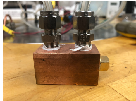
Figure 4.22: Copper block used to help dissipate heat from the inductive circuit
