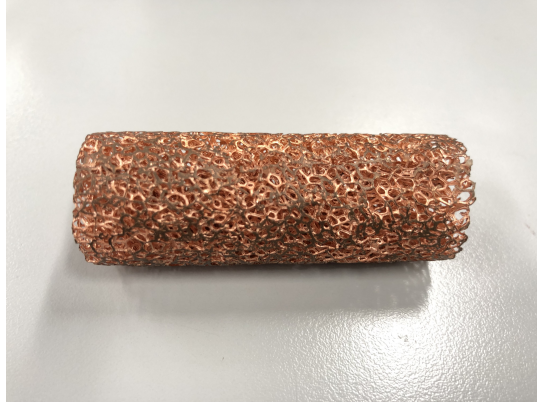
Figure 3.1: Copper metal foam: 0.88 inches diameter, 2.5 inches long
