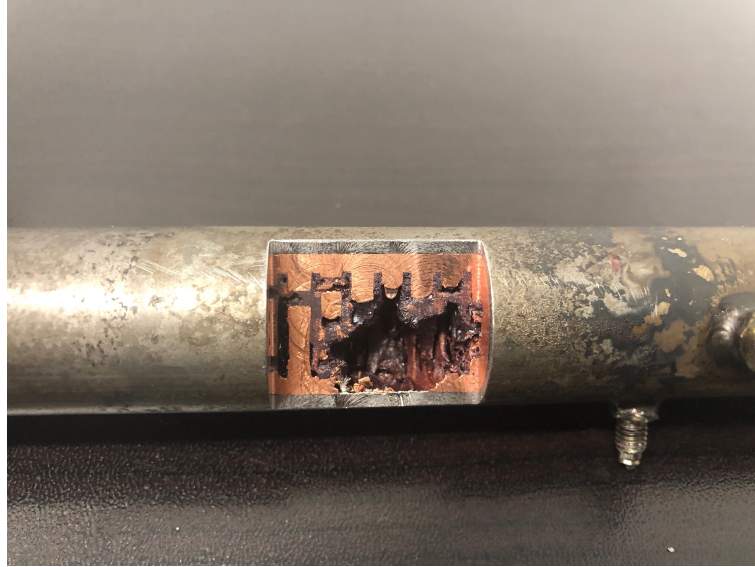
Figure 4.14: Degradation of the copper heat exchanger inside the housing (downstream on right side)
