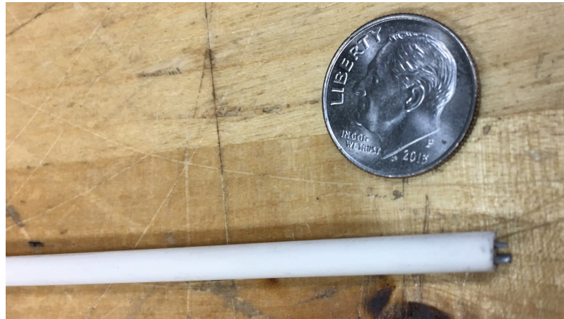
Figure 6.3: Triple Langmuir probe used for helicon and superconducting helicon thruster diagnostic measurements.
