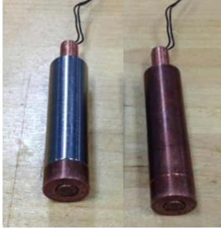
Figure 9: Thermal picks (d) and (e). Titanium insulated pick (e) shown left and uninsulated copper pick (d) shown right.
