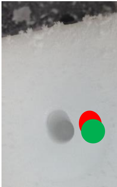
Figure 7: Oblong bore caused by lateral slipping. Visual aid with desired (green) and undesired (red) bore area.
