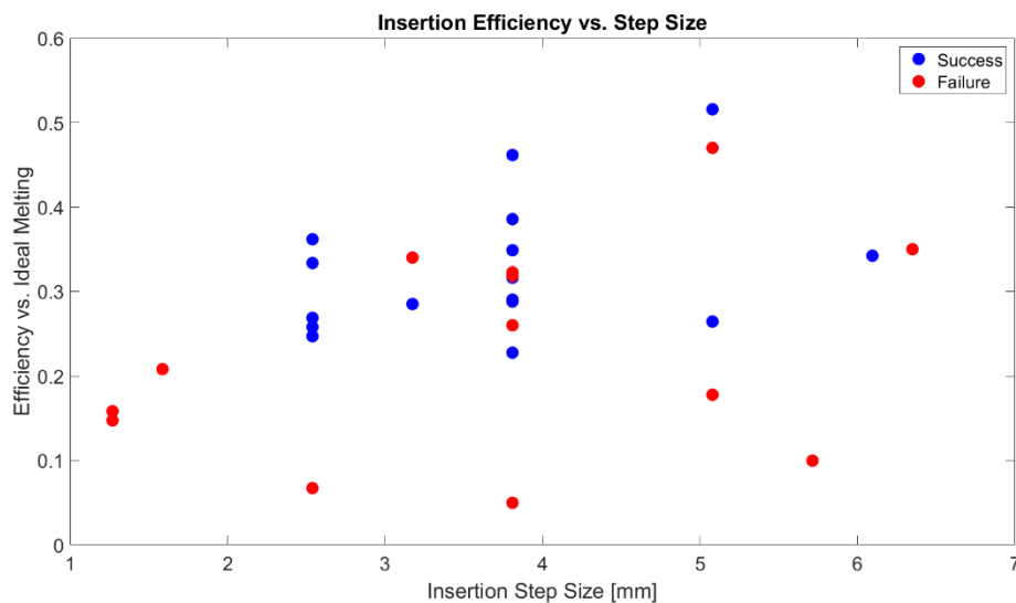
Figure 30: Efficiency relative to ideal melting vs. insertion step size for all water ice insertion tests.
