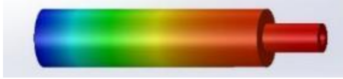
Figure 13: Simulated exposure of thermal pick (d) to a cold reservoir at the thermal pick tip with thermal losses evenly distributed across the walls of the thermal pick.
