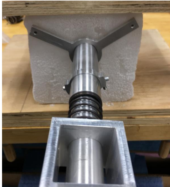
Figure 64: Experimental testing of the long thermal pick end effector bored into cryogenic water ice at atmospheric pressure.
