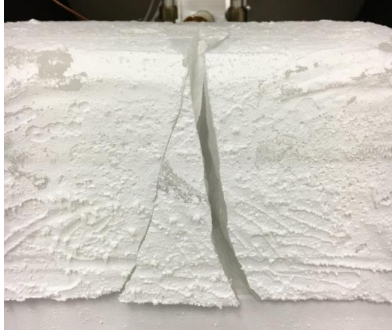
Figure 39: Ice fracture resulting from improper operating conditions. Ice blocks were physically separated so that the extent of the fracture could be seen.
