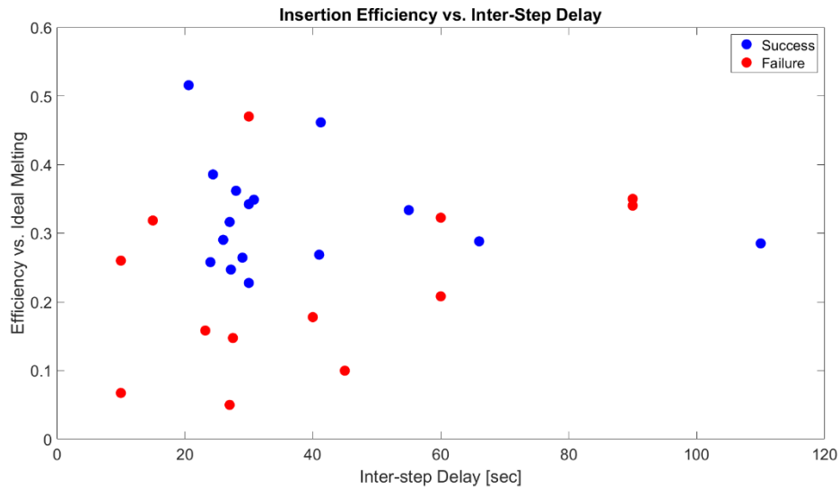
Figure 33: Efficiency relative to ideal melting vs. inter-step delay for all water ice insertion tests.
