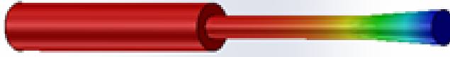
Figure 43: Simulated exposure of thermal pick (A) to a cold reservoir at the tip showing the thermal gradient that forms as a result of heat transfer.
