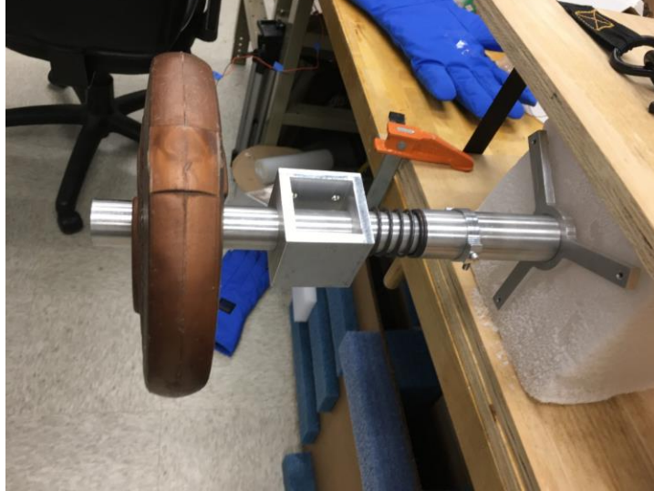
Figure 65: Cantilever loading of the long thermal pick end effector.
