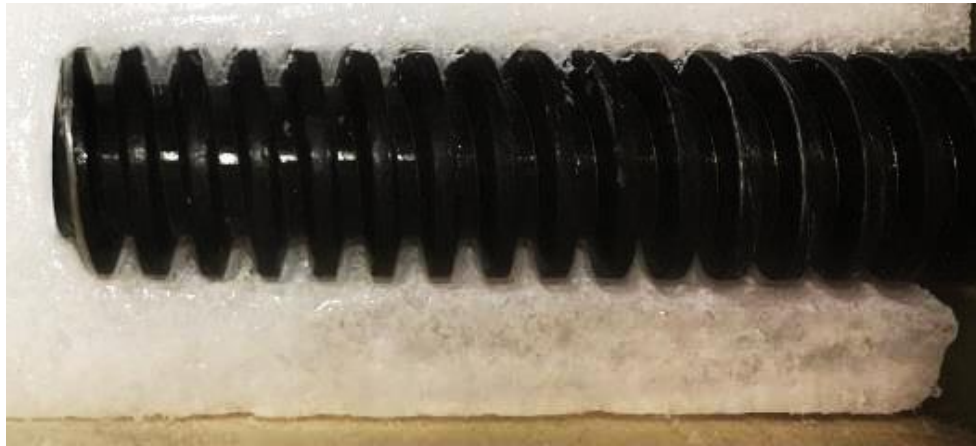
Figure 6: Cross cut of threaded ice borehole and thermal pick (f). Thread quality degrades towards the surface of the ice due to thermal erosion.
