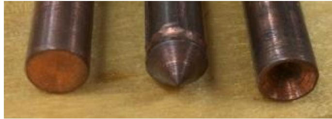
Figure 11: Thermal picks (a), (b), and (c). Flat, conical, and inverse conical tips shown left to right.
