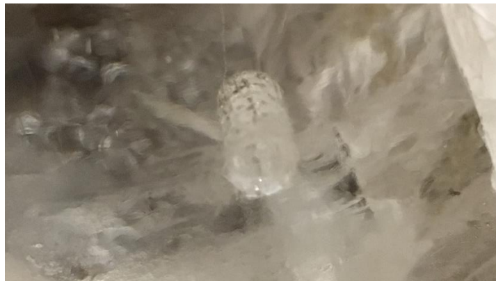
Figure 50: Borehole in optically clear ice using thermal pick (A). Cracks due to thermal shock of test preparation can be seen.
